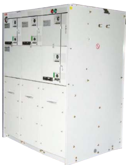
From IAC-test with arc suppressor
